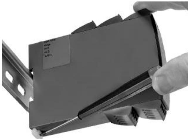
The device is released from the DIN rail by loosening the lower catch.
