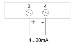
The analog output can be operated actively or passively. Attention: The changeover is only to be carried out in a deenergized state. The electronics can be destroyed.
