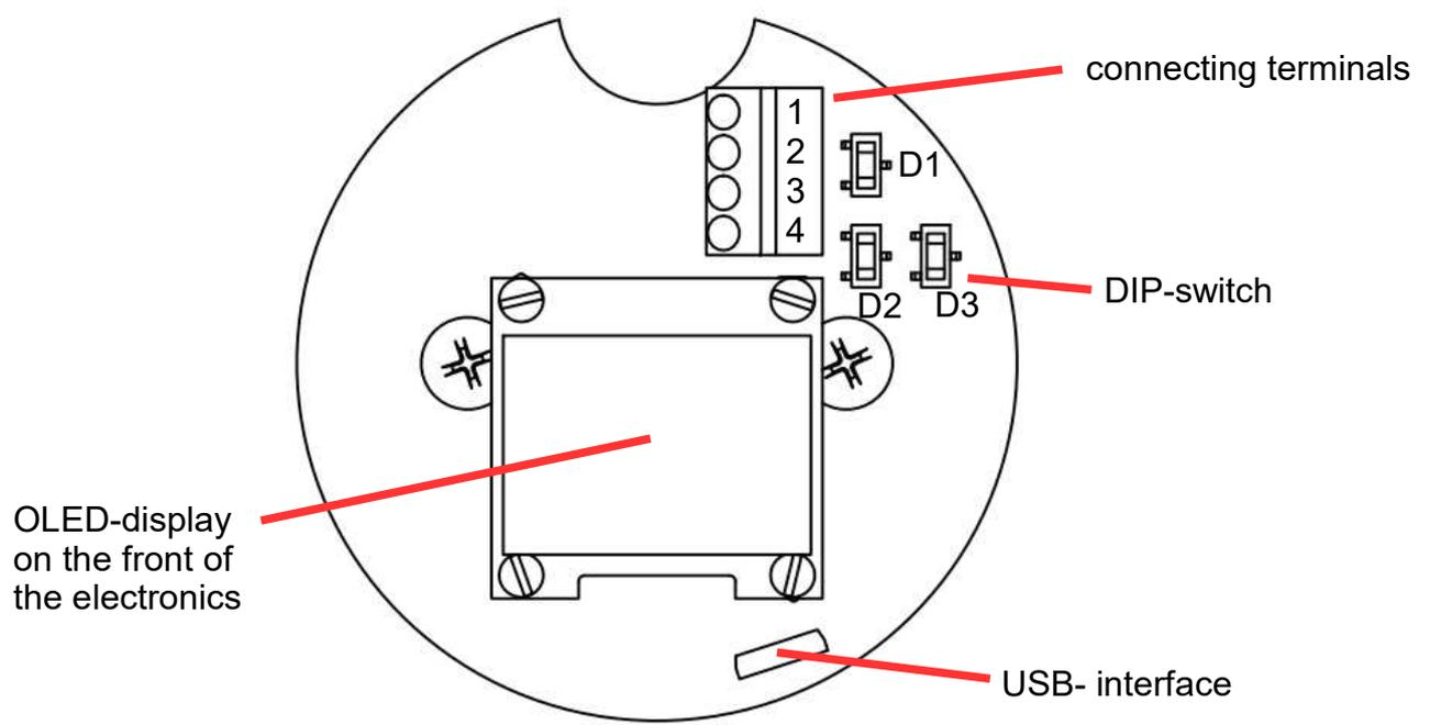
The electronics can be configured via the USB interface. The operating instructions and the software can be found on our homepage for the respective device.
