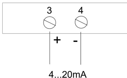
The analog output can be operated actively or passively. Attention: The changeover is only to be carried out in a deenergized state. The electronics can be destroyed.
